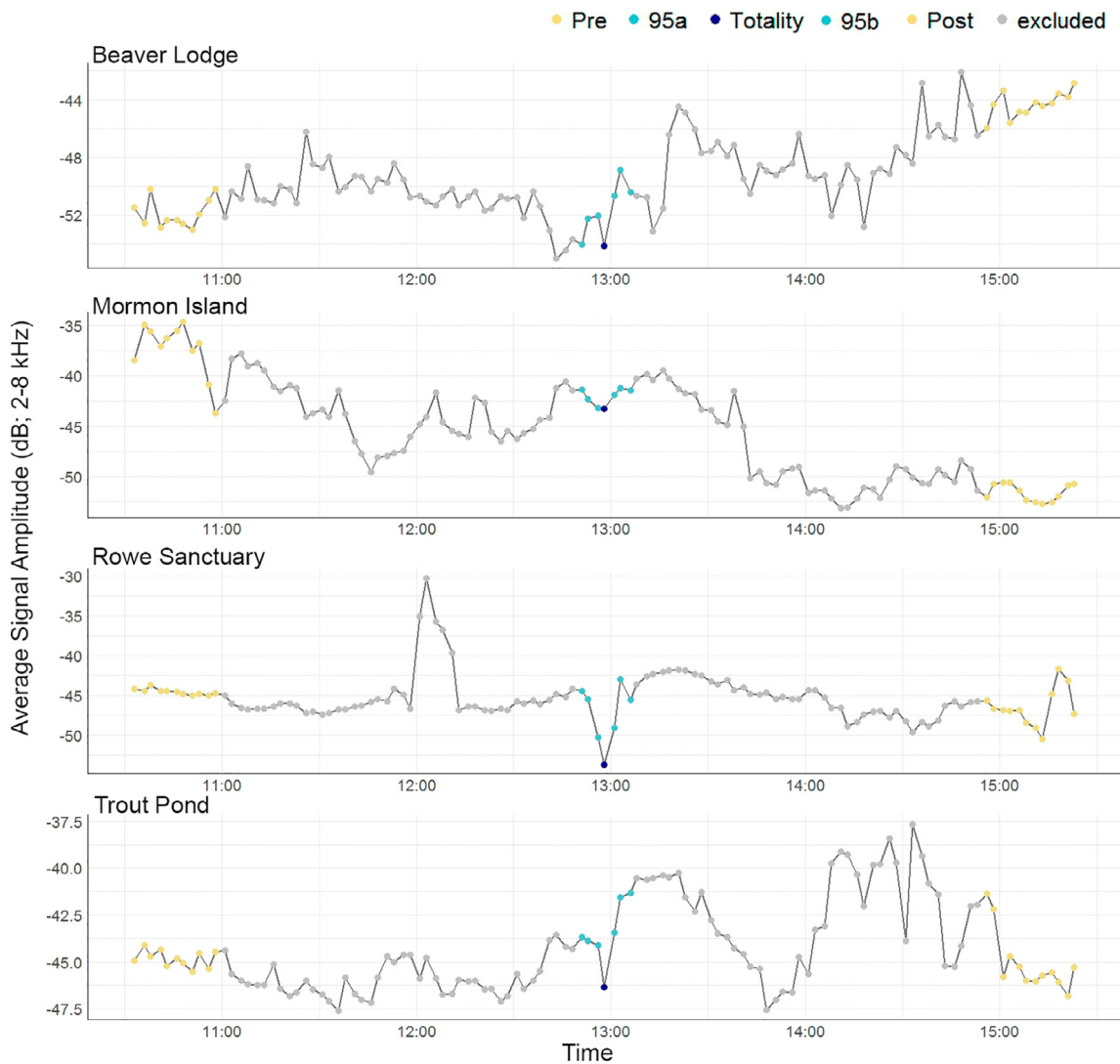
Fig. 10. Average Signal Amplitude (ASA) values plotted from 10:30 to 15:30 on 21 August 2017. ASA, the mean amplitude of the wave envelope based on methods in Towsey et al. (2014), was calculated for 2.5-minute bins in the 2–8 kHz range. Colors designate values within eclipse phases (pre-eclipse, 95%a, totality, 95%b, post-eclipse) used in other analysis.
