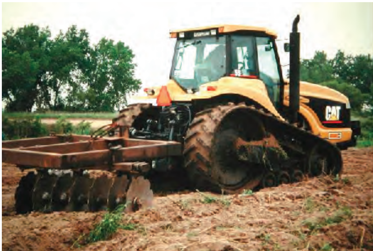
Fig. 3. Caterpillar Challenger rubber-tracked tractor used to maintain open stretches of the Platte River in Nebraska by the Platte River Whooping Crane Maintenance Trust, Inc.
