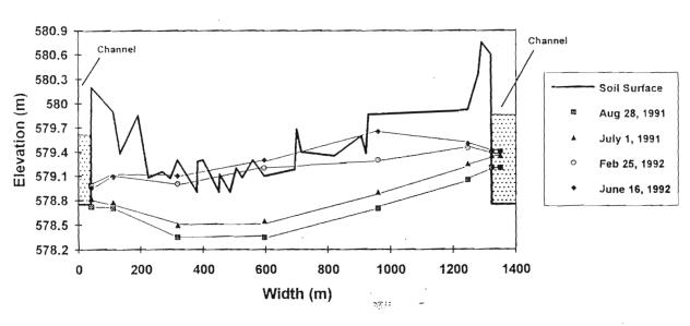
Figure 2. A profile of the surface and groundwater levels at Mormon Island Crane Meadows. Ground water levels fluctuate throughout the year but are generally highest in the spring when precipitation and river stage levels are normally high.
