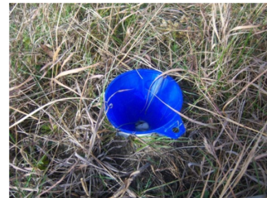
Figure 3. Seed trap made from a plastic funnel and PVC pipe.
