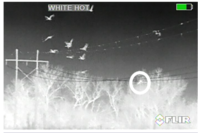
Fig. 8. Sandhill Crane power line collision documented when the Avian Collision Avoidance System was off (white circle) using a Forward Looking InfraRed (FLIR) night vision scope with an attached video recorder.
